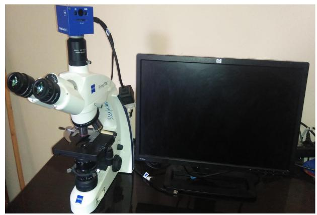
Figure 39: Microscope ZEISS PrimoStar muni d'une camera AxioCam EPc 5s
