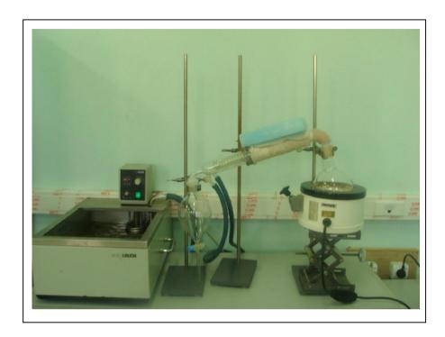
**Photo 01:** Dispositive d'hydro-distillation
