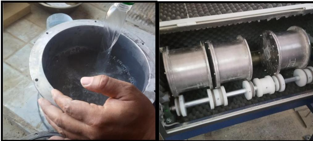
Figure (III. 17) Essai Micro-Deval
