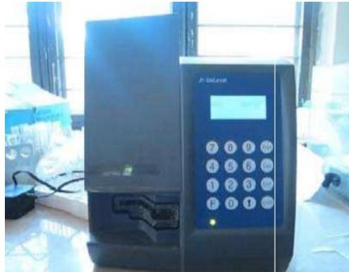
**Figure 06.** Coulter counter (DeLaval) (Reddy et *coll.*, 2014)
