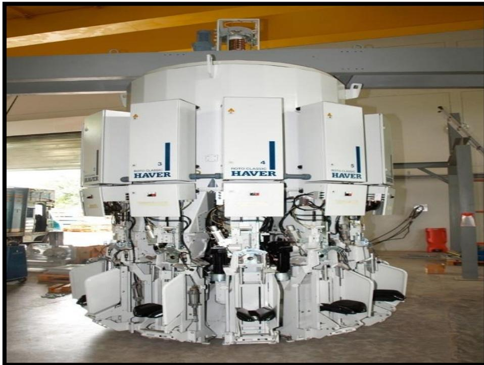
**Figure II.1:** Machine roto-packer type 10RSE
