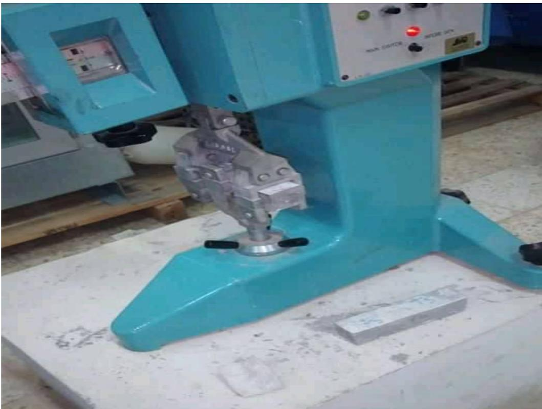
*Figure IV.2 Machine de traction.*
