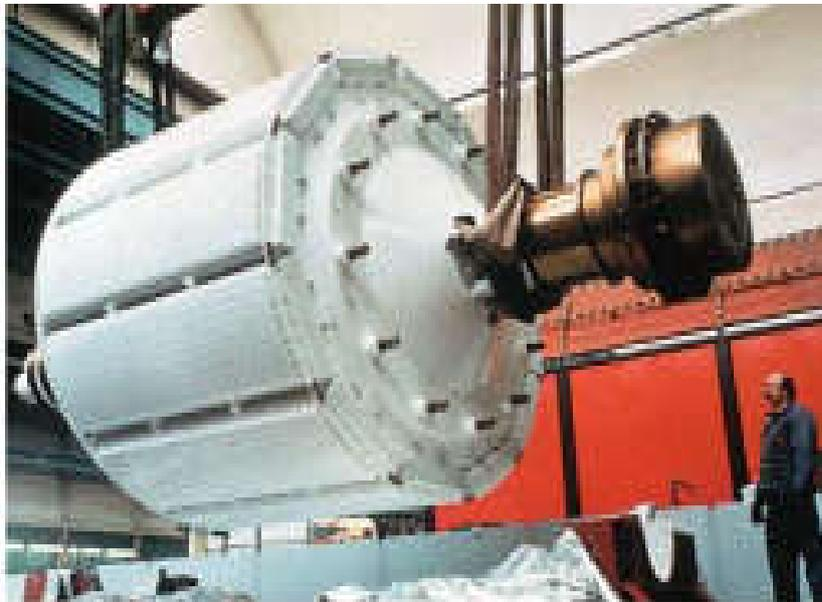
**Fig.I 4** : Machine synchrone 100 MW
