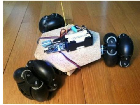
**Figure 1.8 :** Robot mobile omnidirectionnel.
