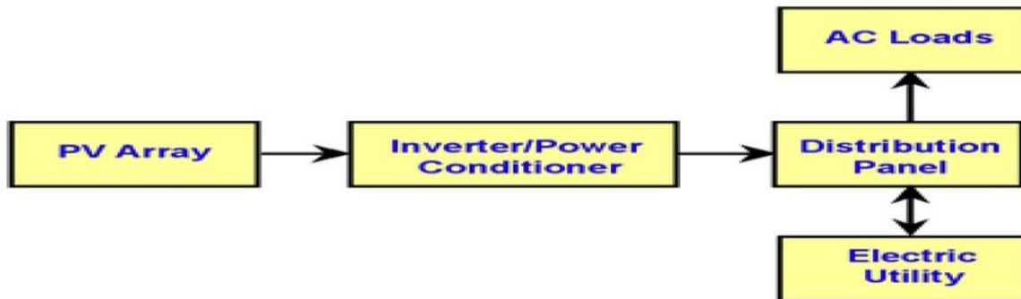
Figure I.10: Grid connected PV system
