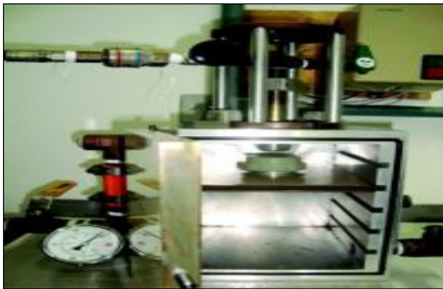
Figure 13.A microparticle accelerator chamber, into which the plant material is placed for the biolistic transformation process. Upon the microparticle's entry into a cell, the attached exogenous DNA dissociates by interaction with cellular fluids and is randomly integrated into the recipient cell genome.
