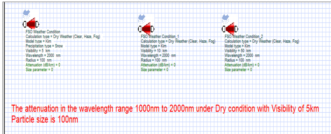
Figure III.16: Attenuation under dry weather conditions for various visibility levels (e.g., clear air, fog, haze). The component uses Mie scattering models (Kim or Kruse) to compute losses based on visibility range.
