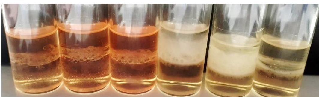
Figure 4. Emulsifying capacity of L. cavernae on diesel oil (left) and gasoline (right).
