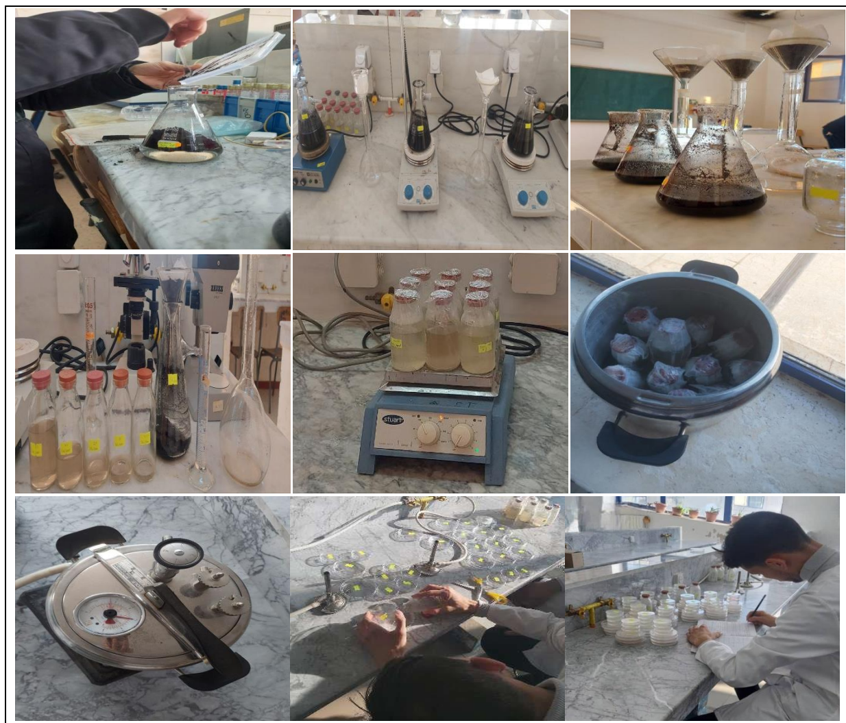
Figure 12 : Steps of Agar-based biochar macerate production.
