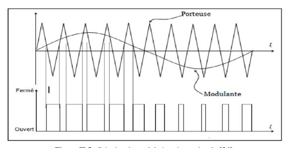
Figure II 5: Principe de modulation sinus-triangle [34].
