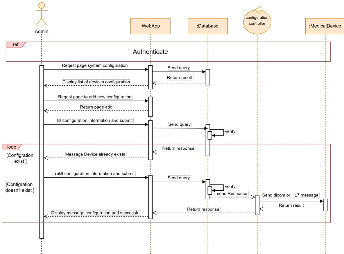
Figure 4.5: System Configuration Sequence Diagram.
