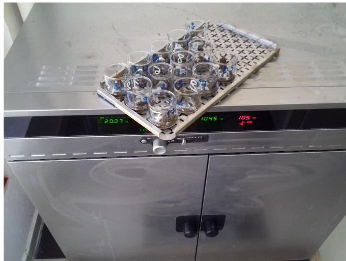
**Figure 21:** Soil moisture by drying technique (O.Bekouider)
