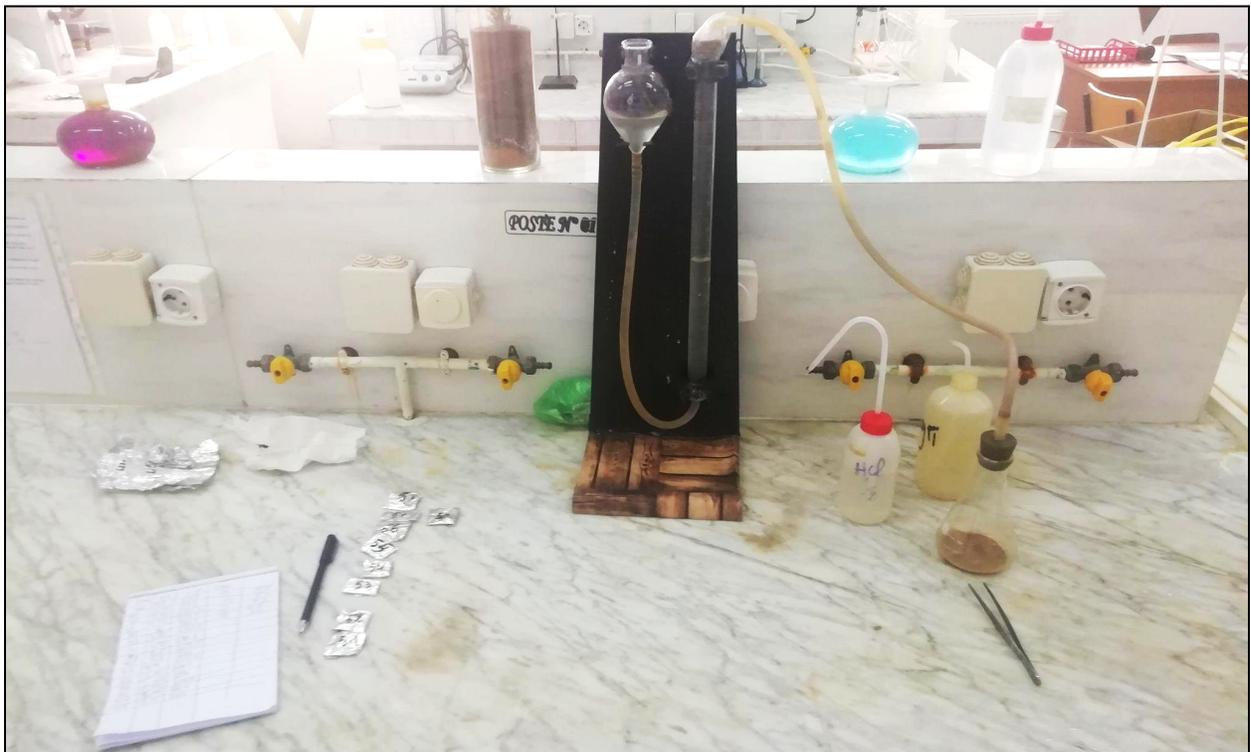
**Figure 26:** TL measurement using the Bernard-calcimeter (O.Bekouider)
