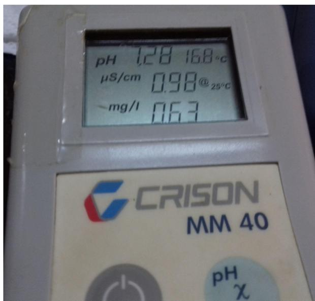
**Figure 25:** EC measurement (O.Bekouider)
