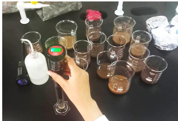
**Figure 22:** NPK Measurements (S.Saadna)
