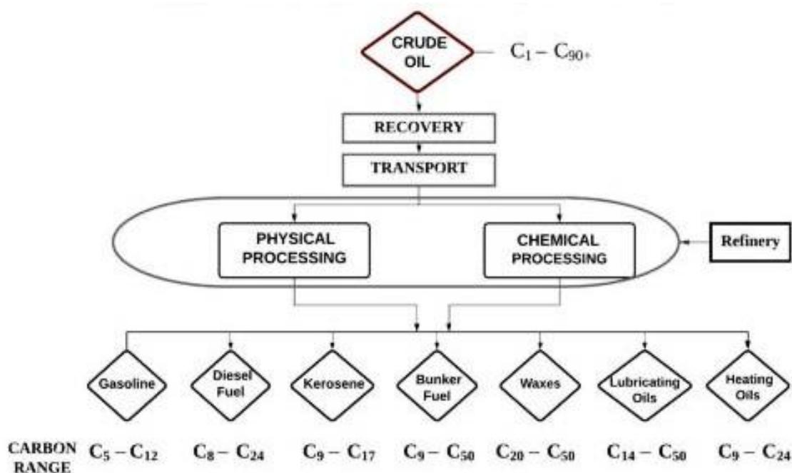
**Figure 1.** Pathways of petroleum hydrocarbons processing (Sayed et al., 2021).
