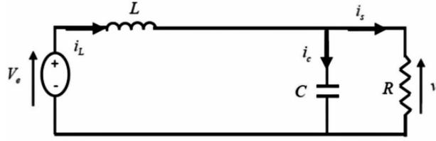
Figure II 14 Boost equivalent circuit when switch is open.
