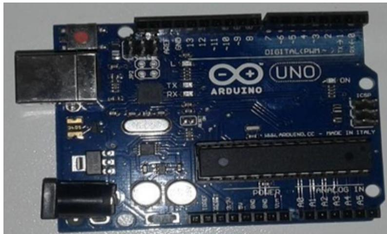
FIGURE 4.4: Arduino UNO board
