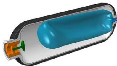
FIGURE 1.7: Hydraulic accumulator
