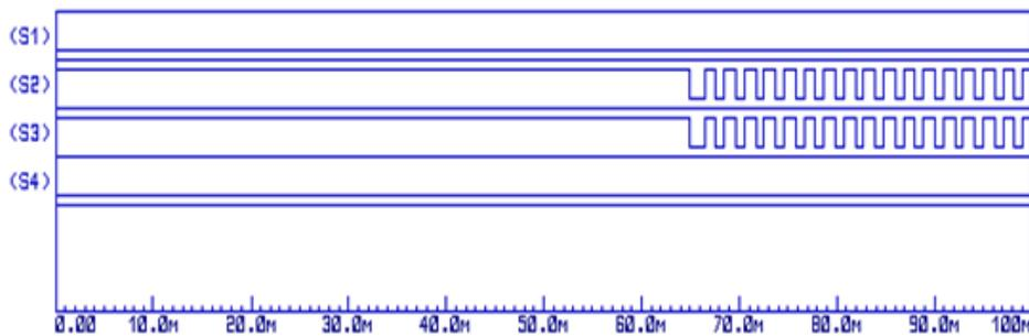
FIGURE 4.15: Control of the switches in backward motoring movement
