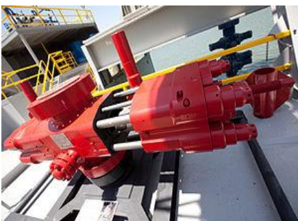
Figure 40: photo of BOP
