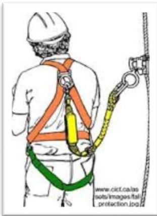
Figure 77: fall arrest system
