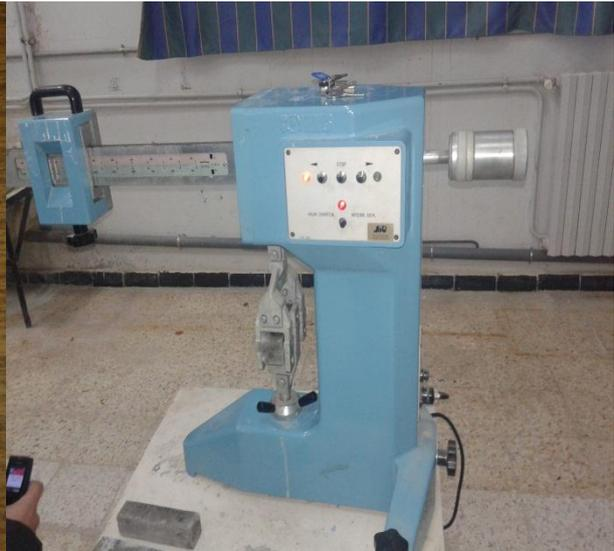
Figure. III.21: Machine de flexion.
