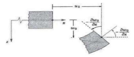
Figure II.9: Illustration de la plaque (CPT)[30].
