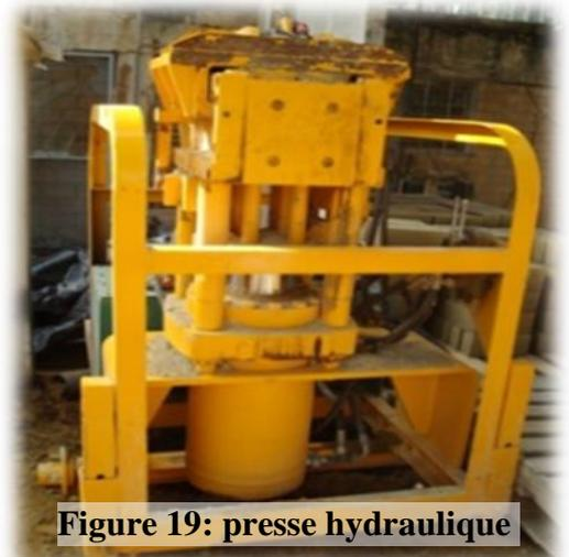
Figure 19: presse hydraulique
